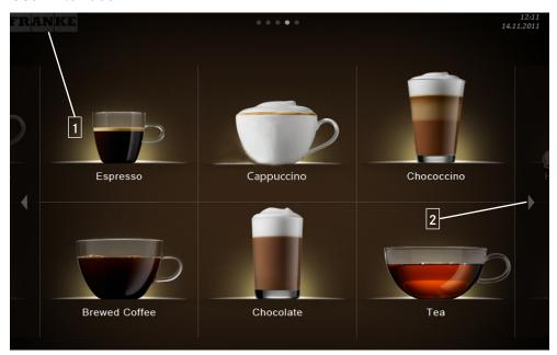
1 The **Franke** button is used to switch between the maintenance level and product selection.
