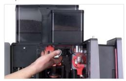
2. Lift and remove the bean hopper.
