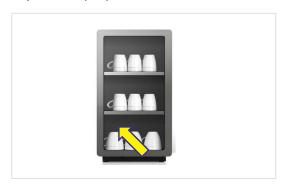
The type plate for the cup warmer is located on the inner side of the rear panel at the bottom left.
