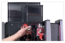
2. Lift and remove the bean hopper.
