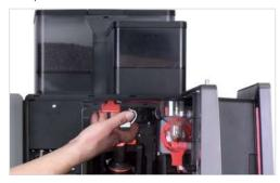
2. Lift and remove the powder hopper.
