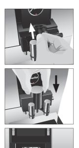
► Fit the assembled individual parts back in the dual spout and press it firmly.
